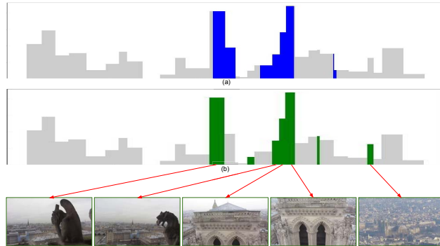
Fig. 2. Visualization 2 of ground truth shot scores (grey), (a) ground truth summary (blue), (b) model generated summary (green) for the video “Notre_Dame” in SumMe dataset.
